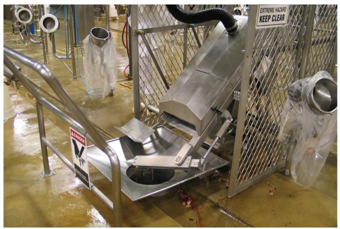
The Jarvis Model AHD-1 Automatic Head Dropper -for continuous sheep head dropping operations on the kill floor.
